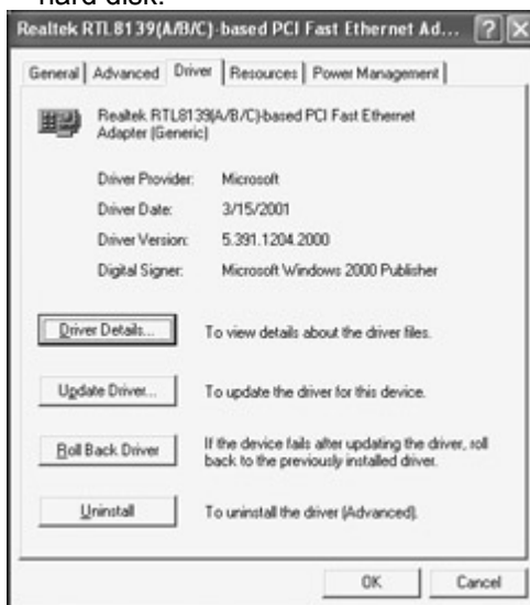
Figure 17-13: The Driver tab in the Properties dialog box for an installed device
