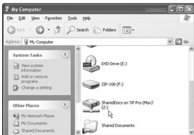
Figure 21-12: A network drive, Z:, mapped to the Shared Documents folder on a computer named Max
