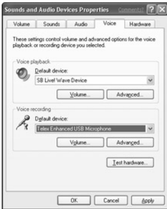
Figure 24-4: The Voice tab of the Sounds and Audio Devices Properties dialog box
