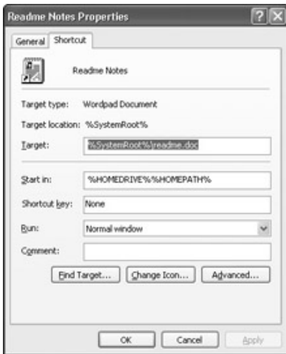
Figure 30-6: The Change Icon button also appears on the Shortcut tab of the Properties sheet.
