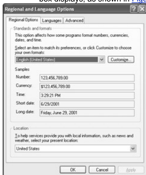
Figure 14-16: Use the Regional Settings Properties dialog box to customize numeric, currency, time, and date formats for your region.
