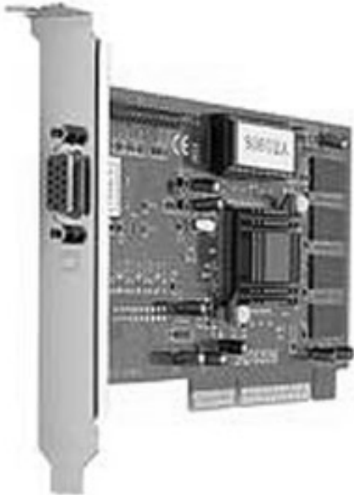
Figure 17-6: A sample card that plugs into an expansion slot. Only the port facing you is visible from outside the computer.
