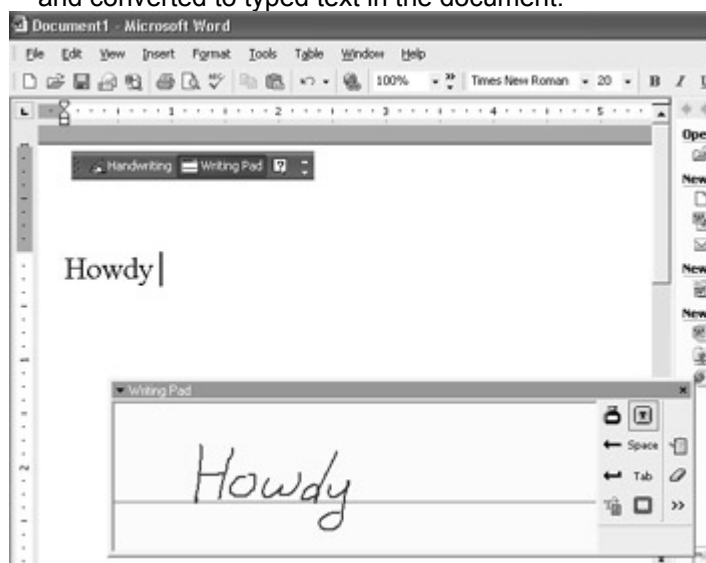
Figure 15-16: The handwritten word “Howdy” converted to typed text in a Word 2002 document
