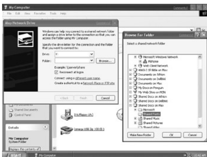
Figure 28-6: Mapping a drive letter to the Shared Fonts folder on the computer named Max from a different computer in the LAN
