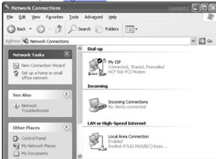
Figure 21-7: On the host computer, the icon for a direct cable connection appears as an Incoming Connections icon.
