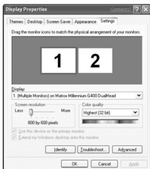
Figure 34-3: The Settings tab of Display Properties with two monitors attached to a dual-head graphics card. One monitor will act as the primary monitor that displays the logon screen and taskbar. You can make either monitor the primary monitor by selecting it and then choosing the “Use this device as the primary monitor” check box. If you have any problems getting multiple monitors to work, try the Troubleshooter. Just click the Troubleshoot button on the Settings tab in the Display Properties dialog box to get started.
