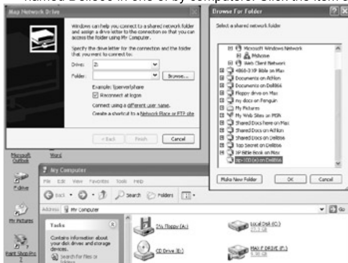
Figure 28-3: Mapping a network drive in My Computer on one machine to a shared Zip drive on another machine
