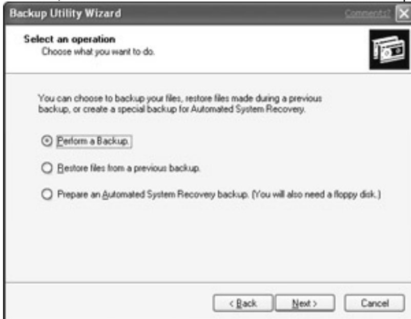
Figure 18-7: This wizard page provides access to the three main capabilities of the Microsoft Backup utility.
