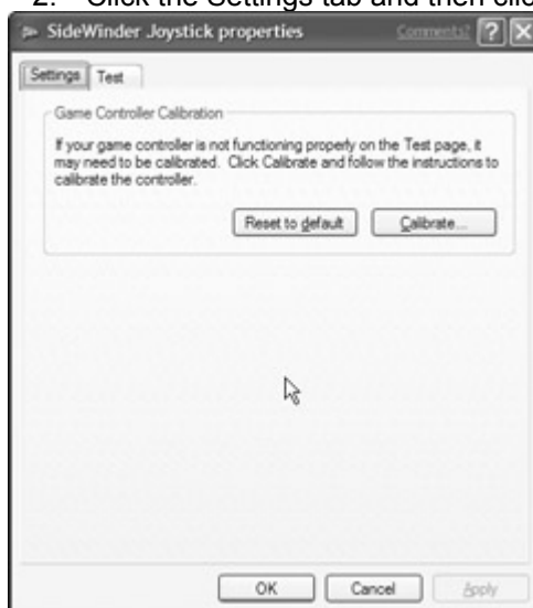
Figure 15-9: Use the Calibrate button to tune your game controller to your PC.
