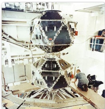
The Vela-5A/B Satellite in its cleanroom. The two satellites, A and B, were separated after launch.
