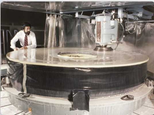
Grinding of Hubble's primary mirror at Perkin-Elmer, March 1979
