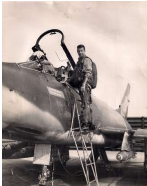
AUTHOR AND HIS F-100 IN A REVETMENT AT BIEN HOA AIR BASE. NOTE 500LB MK-82 SNAKE EYE BOMB WITH FOLDING FINNS UNDER WING.
