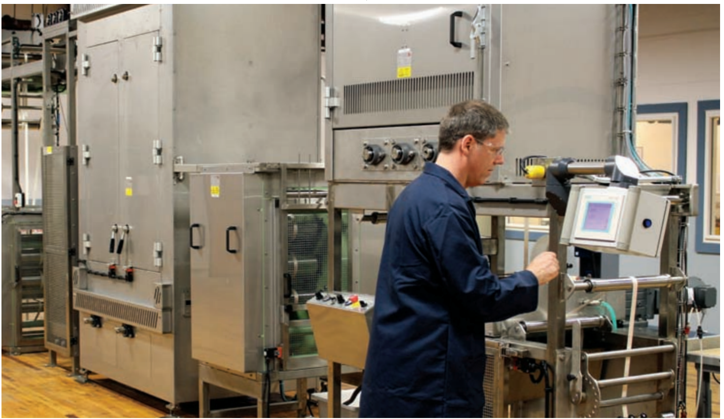
❖ Above: A technician applies an abrasion treatment to a webbing.
