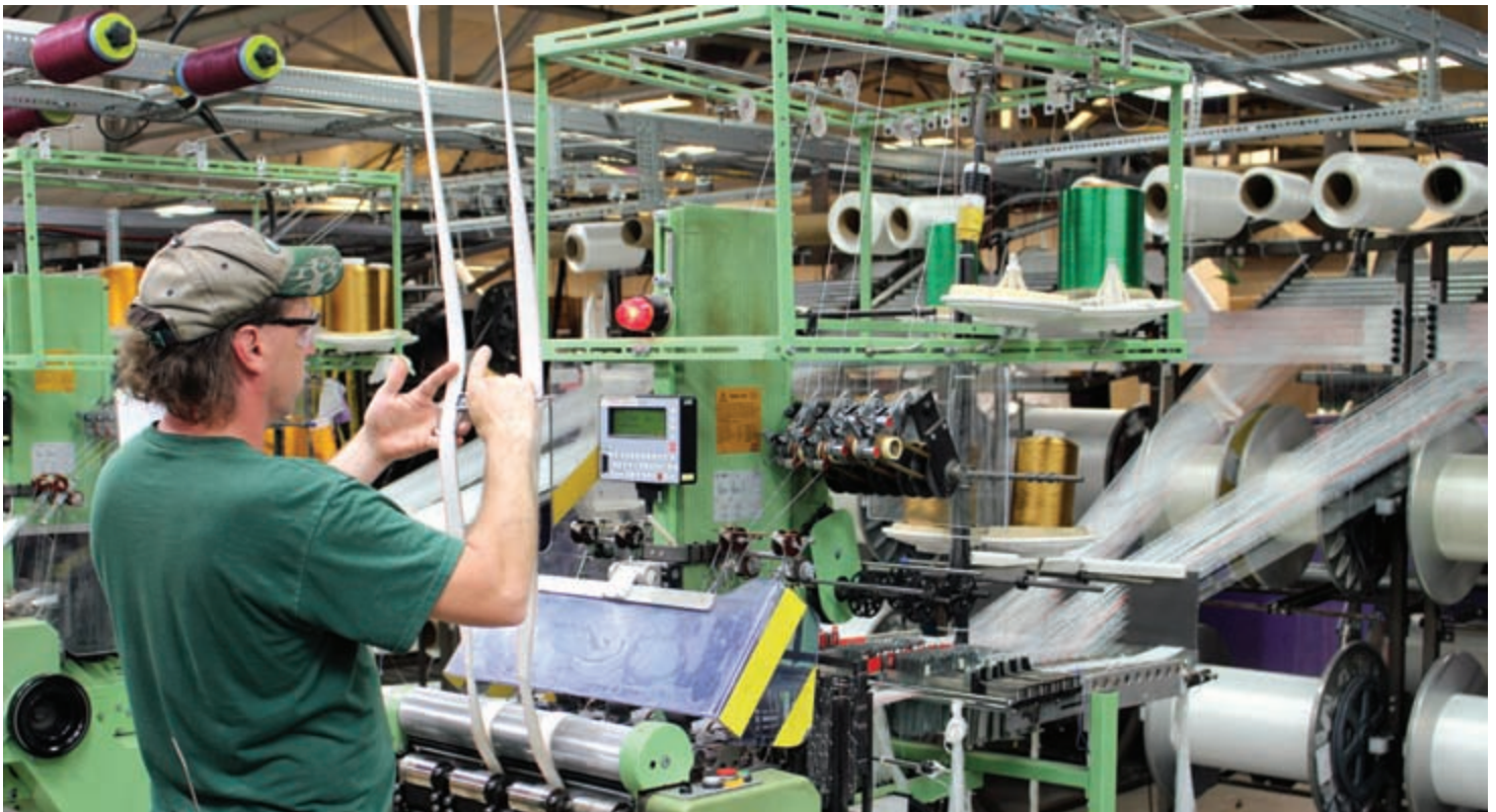
Below: A weaving technician checks the width of a webbing at a needle loom.
