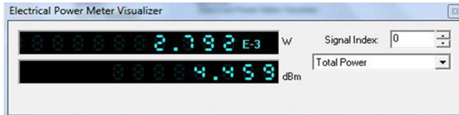
Fig. 7 Electrical Power Output (With 3dBm Injection)
