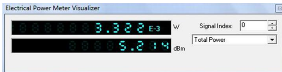
Fig. 8 Electrical Power Output (With 4dBm Injection)
