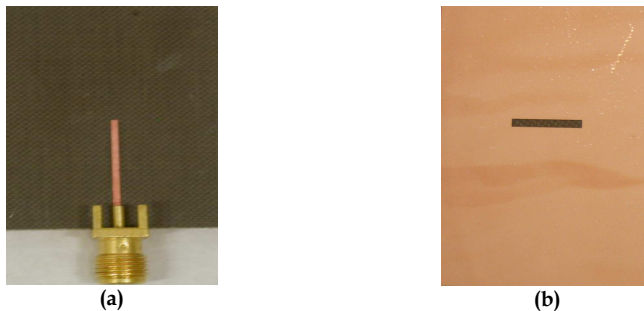
Fig. 18. Optical images of (a) a feeding microstrip and (b) a coupling aperture on a substrate after fabrication.
