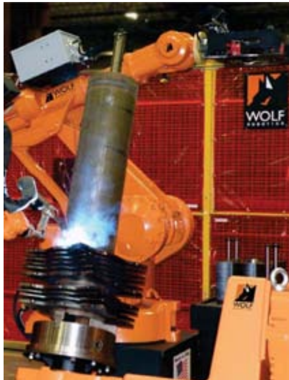
Below: Robotic welding system producing chopping blades for agricultural equipment manufacturer.
