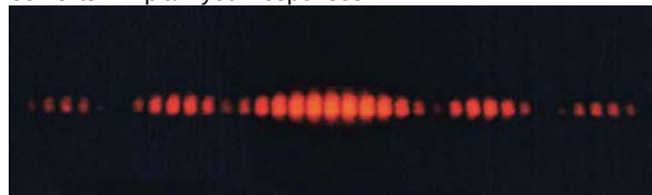
Figure 27.55 This double slit interference pattern also shows signs of single slit interference. (credit: PASCO)
