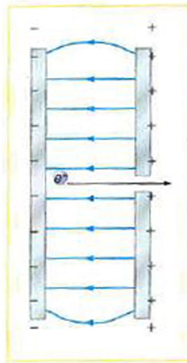
Figure 18.55 Parallel conducting plates with opposite charges on them create a relatively uniform electric field used to accelerate electrons to the right. Those that go through the hole can be used to make a TV or computer screen glow or to produce X-rays.
