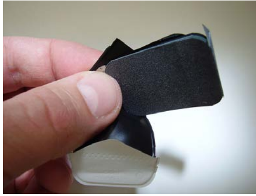
Figure 31.8 Film badges contain film similar to that used in this dental x-ray film and is sandwiched between various absorbers to determine the penetrating ability of the radiation as well as the amount. (credit: Werneuchen, Wikimedia Commons)
