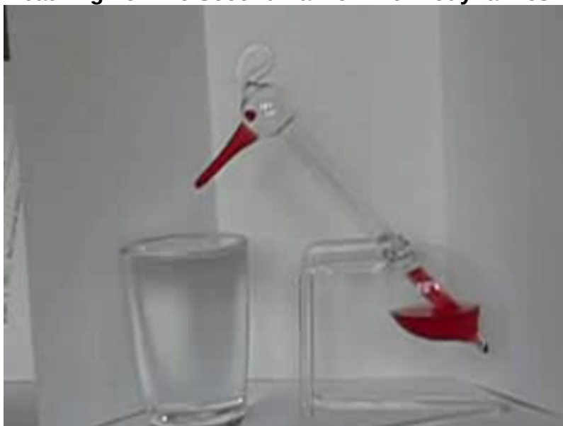
Figure 15.21 This novelty toy, known as the drinking bird, is an example of Carnot's engine. It contains methylene chloride (mixed with a dye) in the abdomen, which boils at a very low temperature—about 100^{\circ}\text{F} . To operate, one gets the bird's head wet. As the water evaporates, fluid moves up into the head, causing the bird to become top-heavy and dip forward back into the water. This cools down the methylene chloride in the head, and it moves back into the abdomen, causing the bird to become bottom heavy and tip up. Except for a very small input of energy—the original head-wetting—the bird becomes a perpetual motion machine of sorts. (credit: Arabesk.nl, Wikimedia Commons)
