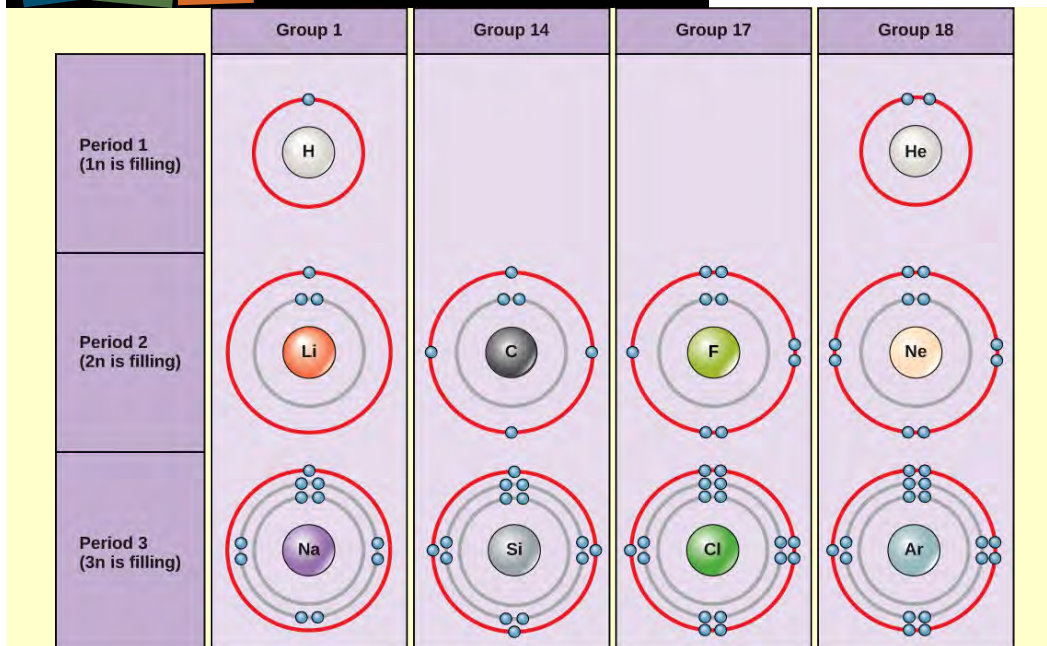
Figure 2.7 Bohr diagrams indicate how many electrons fill each principal shell. Group 18 elements (helium, neon, and argon are shown) have a full outer, or valence, shell. A full valence shell is the most stable electron configuration. Elements in other groups have partially filled valence shells and gain or lose electrons to achieve a stable electron configuration.
