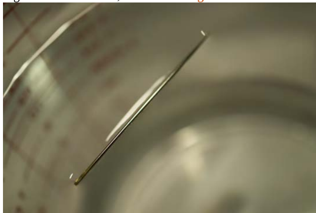
Figure 2.16 The weight of the needle is pulling the surface downward; at the same time, the surface tension is pulling it up, suspending it on the surface of the water and keeping it from sinking. Notice the indentation in the water around the needle. (credit: Cory Zanker)
