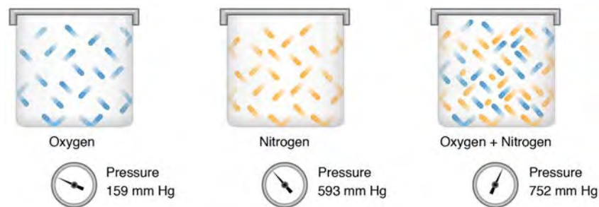
Figure 22.21 Partial and Total Pressures of a Gas Partial pressure is the force exerted by a gas. The sum of the partial pressures of all the gases in a mixture equals the total pressure.
