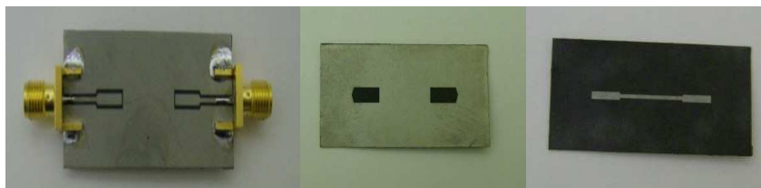
Fig. 6. Photograph of the fabricated UWB filter.
